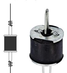
The **RSIC-WHI** is designed for use with any wood, steel or concrete application where a dropped drywall ceiling is required. The RSIC-WHI isolator installed mid-wire between the structure and a drywall grid ceiling, or CRC and hat channel ceiling. The RSIC-WHI Isolator has acoustical design load ratings of 30, 50, 70, 100, 145, and 220 lbs per isolator.
