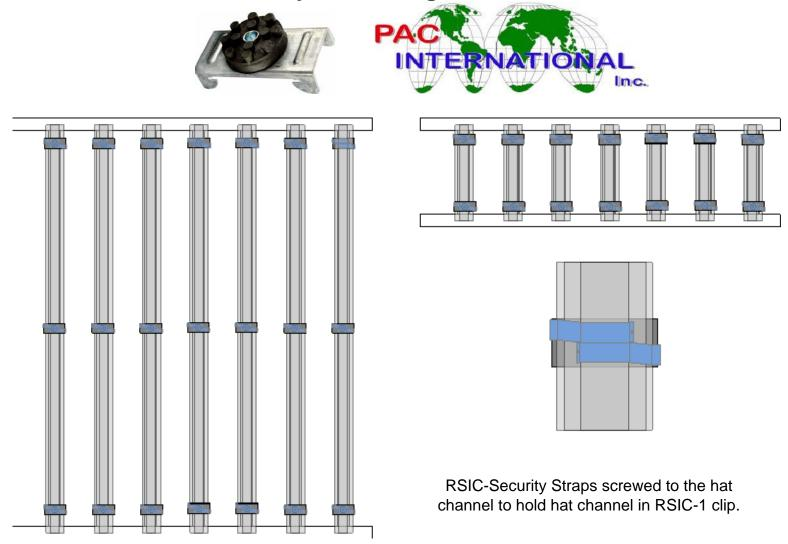
Hat channel snapped into RSIC-1 clips and secured with RSIC-Security Straps and Fasteners through the hat channel to keep the hat channel from sliding within the RSIC-1 clips
